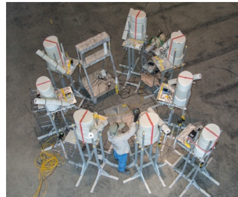
Testing handheld neutron detectors for the Backpack, Handheld, and Vehicle Mounted Neutron Detection Replacement Program
