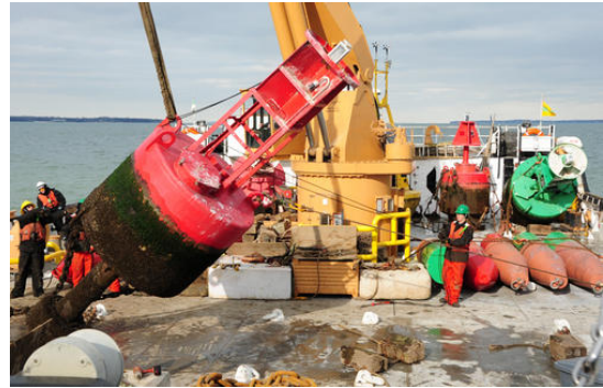
Lake Erie – The crew of Coast Guard Cutter BRISTOL BAY, removing a buoy in Nov 2012 as part of District 9's annual "Fall Retrieve", which is designed to limit damage to AToN in the winter months.
