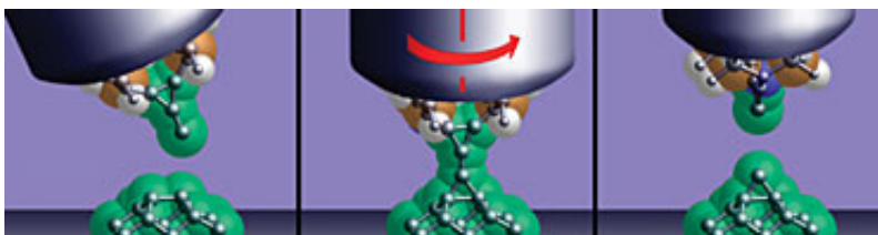
MECHANOSYNTHETIC REACTIONS As conceived by Drexler, to deposit carbon, a device moves a vinylidenecarbene along a barrier-free path to insert into the strained alkene, twists 90° to break a pi bond, and then pulls to cleave the remaining sigma bond. COURTESY OF K. ERIC DREXLER
